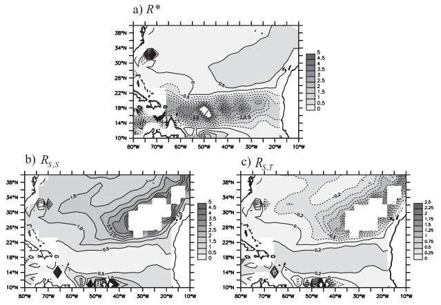
FIG. 9. (a) Annual mean density ratio  $R^*$  (unitless). (b) Annual mean coefficient  $R_{S,S}$  (unitless). (c) Annual mean coefficient  $R_{S,T}$  (unitless). Regions where  $R^*$  is between 0.8 and 1.2 are masked in (b) and (c). See the text.
