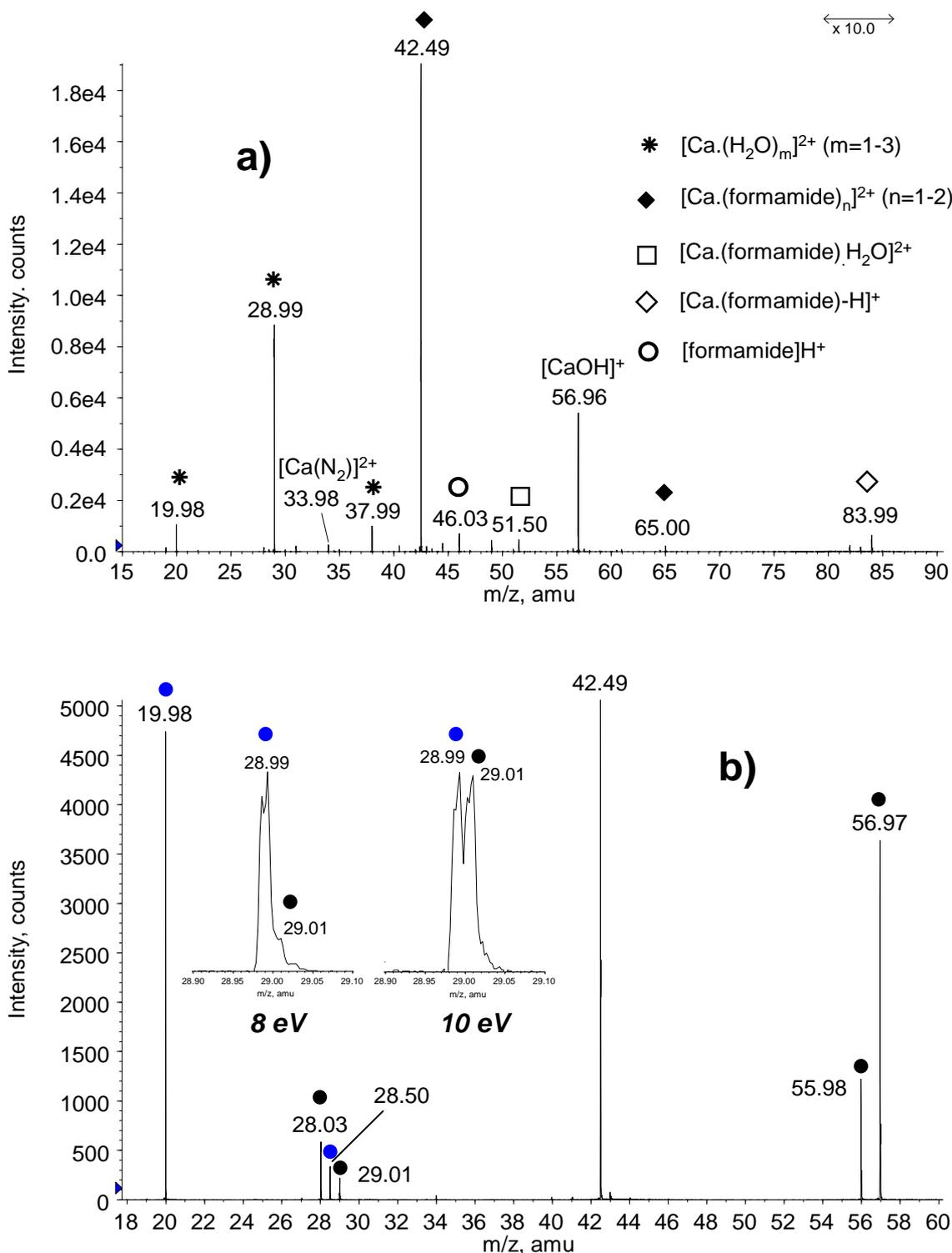
Figure 1: **a)** Positive nanoelectrospray spectrum of an aqueous CaCl<sub>2</sub>/formamide ( $10^{-3}$  mol L<sup>-1</sup>/ $10^{-4}$  mol L<sup>-1</sup>) mixture, recorded with a declustering potential of 20 V; **b)** Low-energy CID spectra of the [Ca(formamide)]<sup>2+</sup> complex recorded with a collision energy of 11 eV (laboratory frame), except the insert. See text for details
