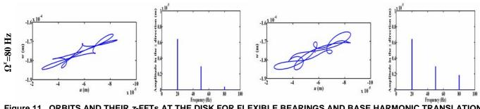
Figure 11. ORBITS AND THEIR z-FFTs AT THE DISK FOR FLEXIBLE BEARINGS AND BASE HARMONIC TRANSLATION  $(Z_0=5\times10^{-5}~\text{AND}~\Omega^z=50~\text{Hz})$ , COMBINED WITH TWO AMPLITUDES OF BASE HARMONIC ROTATIONS:  $\omega^{x,a}=(a)~10^{-2}~\text{rad/s},~(b)~5\times10^{-2}~\text{rad/s},~(\Omega^x=20~\text{Hz},~50~\text{Hz}~\text{AND}~80~\text{Hz})$
