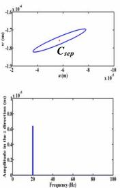
Figure 8. MASS UNBALANCE ORBIT AND ITS z-FFT AT THE DISK FOR FLEXIBLE BEARINGS AND FIXED BASE
