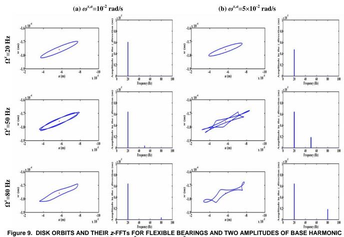
ROTATIONS:  $\omega^{x,a}$  = (a)  $10^{-2}$  rad/s, (b)  $5 \times 10^{-2}$  rad/s, ( $\Omega^{x}$  = 20 Hz, 50 Hz AND 80 Hz)
