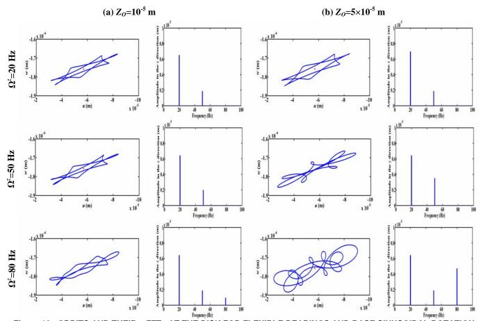
Figure 10. ORBITS AND THEIR z-FFTs AT THE DISK FOR FLEXIBLE BEARINGS AND BASE SINUSOIDAL ROTATION ( $\omega^{x,a}$ =5×10<sup>-2</sup> rad/s AND  $\Omega^x$ =50 Hz), COMBINED WITH TWO AMPLITUDES OF BASE SINUSOIDAL TRANSLATIONS:  $Z_{O}$ = (a) 10<sup>-5</sup> m, (b) 5×10<sup>-5</sup> m, ( $\Omega^z$ =20 Hz, 50 Hz AND 80 Hz)
