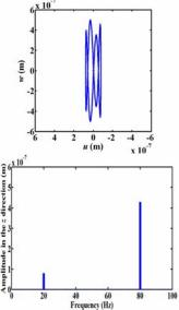
Figure 7. DISK ORBIT AND ITS z-FFT FOR RIGID BEARINGS AND BASE HARMONIC ROTATION:  $\omega^{x,a}$ =5×10<sup>-2</sup> rad/s AND  $\Omega^x$ =80 Hz
