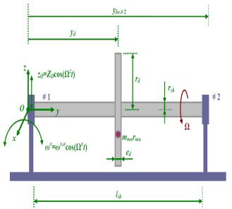
Figure 5. ON-BOARD ROTOR-BEARING SYSTEM CONFIGURATION
