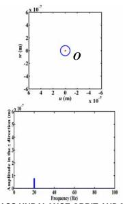
Figure 6. MASS UNBALANCE ORBIT AND ITS z-FFT AT THE DISK FOR RIGID BEARINGS AND FIXED BASE
