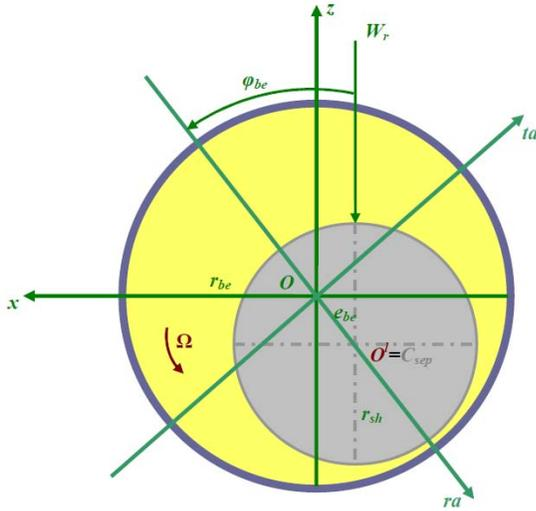
Figure 3. SCHEMATIC VIEW OF A HYDRODYNAMIC BEARING
