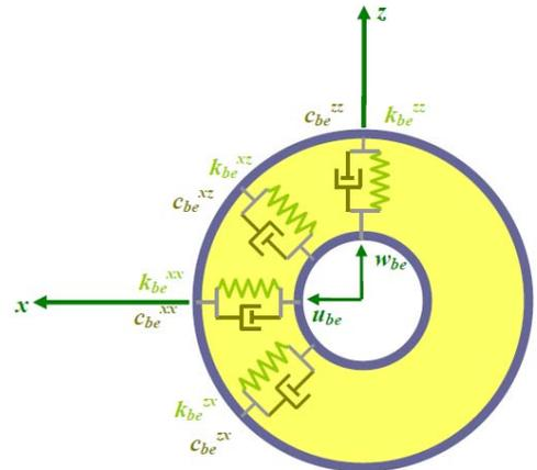
Figure 4. BEARING DAMPING AND STIFFNESS COEFFICIENTS
