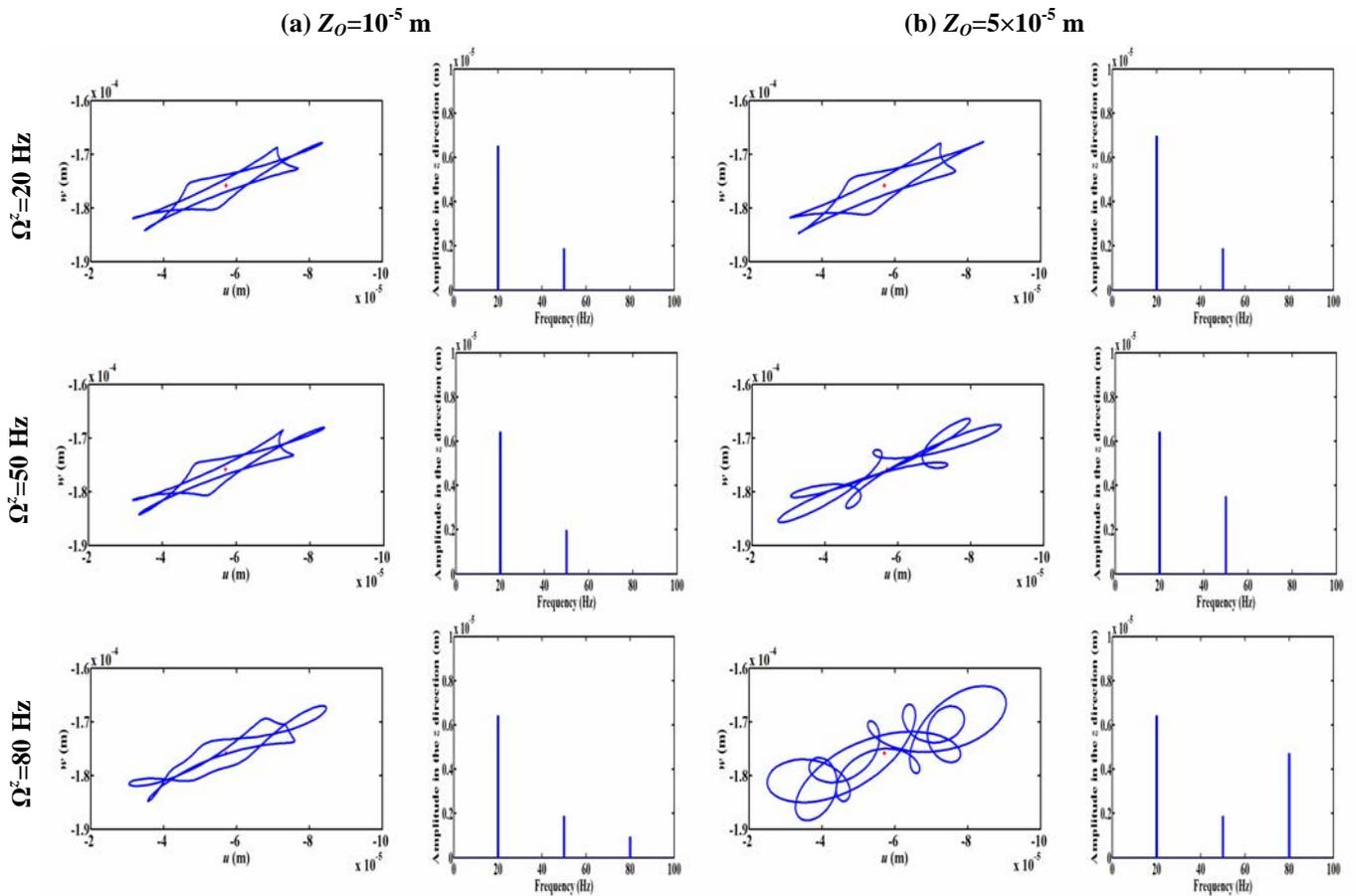
Figure 10. ORBITS AND THEIR z-FFTs AT THE DISK FOR FLEXIBLE BEARINGS AND BASE SINUSOIDAL ROTATION ( $\omega^{x,a}=5 \times 10^{-2}$  rad/s AND  $\Omega^x=50$  Hz), COMBINED WITH TWO AMPLITUDES OF BASE SINUSOIDAL TRANSLATIONS:  $Z_0$ = (a)  $10^{-5}$  m, (b)  $5 \times 10^{-5}$  m, ( $\Omega^z=20$  Hz, 50 Hz AND 80 Hz)
