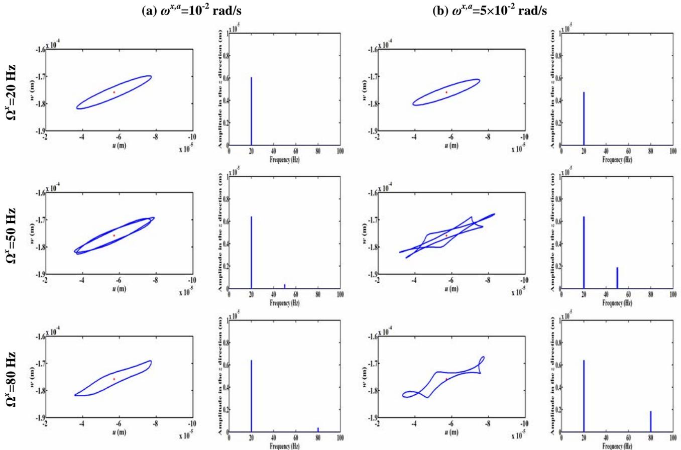
Figure 9. DISK ORBITS AND THEIR  $z$ -FFTs FOR FLEXIBLE BEARINGS AND TWO AMPLITUDES OF BASE HARMONIC ROTATIONS:  $\omega^{x,a} =$  (a)  $10^{-2}$  rad/s, (b)  $5\times 10^{-2}$  rad/s, ( $\Omega^x=20$  Hz, 50 Hz AND 80 Hz)
