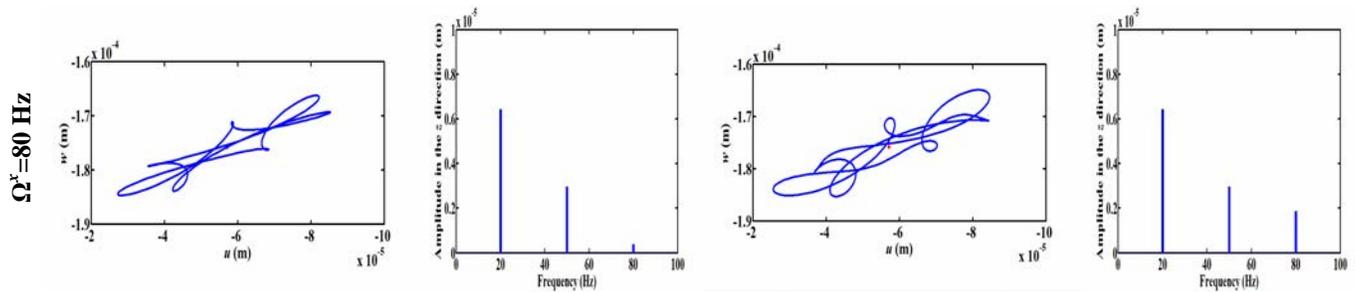
Figure 11. ORBITS AND THEIR z-FFTs AT THE DISK FOR FLEXIBLE BEARINGS AND BASE HARMONIC TRANSLATION ( $Z_0=5 \times 10^{-5}$  AND  $\Omega^z=50$  Hz), COMBINED WITH TWO AMPLITUDES OF BASE HARMONIC ROTATIONS:  $\omega^{x,a} =$  (a)  $10^{-2}$  rad/s, (b)  $5 \times 10^{-2}$  rad/s, ( $\Omega^x=20$  Hz, 50 Hz AND 80 Hz)
