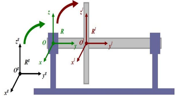
Figure 1. REFERENCE FRAMES OF THE ON-BOARD ROTOR
