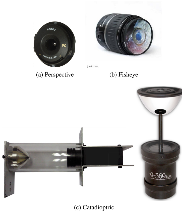
Figure 2: Perspective and omnidirectional (Fisheye and Catadioptric) cameras
