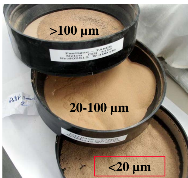
Fig. 5. Soil collected on the three stages of the dry sieving column at the end of the fine particle production process. The relative colors are indicative of the respective content: the upper stage ( 100\text{-}\mu\text{m} mesh) retains small organic debris (black grains), the largest sand grains and possibly clay aggregates; the intermediate stage ( 20\text{-}\mu\text{m} mesh) which contains about 3/4 of the total mass contains mostly the fine, orange-yellowish colored, sand mode and a fraction of aggregated clay; the bottom stage contains the light brown-yellowish, finest fraction of disaggregated particles, dominated by clay (photo F. Dulac).
