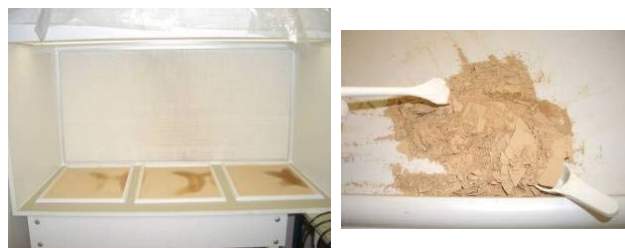
Fig. 6. Artificial aging of the atmospheric particles. The principle is to quickly evaporate a water-aerosol mixing in the typical proportions of a cloud drop that is deposited on ultraclean polypropylene plates under clean air within a laminar flow bench. Water is amended with substances normally observed in Mediterranean marine atmosphere. The added aerosols are the finest fractions of the dust collected in Tunisia. The evaporation leads to a pH gradient in the system induced by proton concentration related to decrease in water volume, exactly as it occurs inside a cloud (photo S. Tran).
