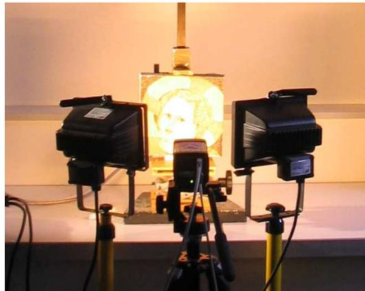
Figure 11: The experimental device implemented for depth measurement of the defect
