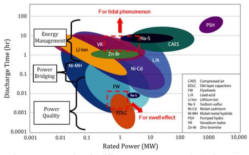
Fig. 16. System ratings for different energy storage technologies [35].
