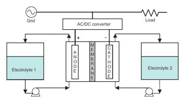
Fig. 9. Flow battery system [10].
