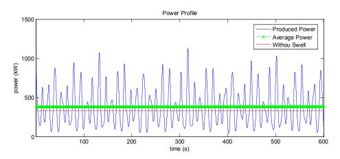
Fig. 6. Power profile of a marine current turbine.
