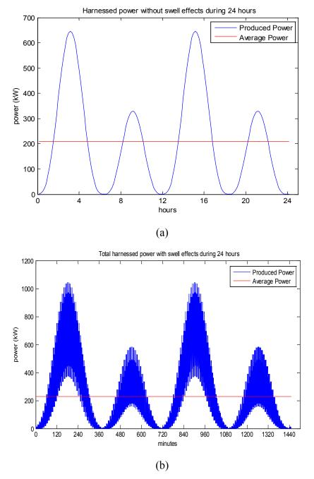
Fig. 1. Power produced by a MCT: (a) without swell, (b) with swell.
