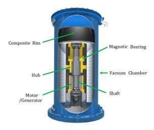
Fig. 10. Typical flywheel energy storage system [15].
