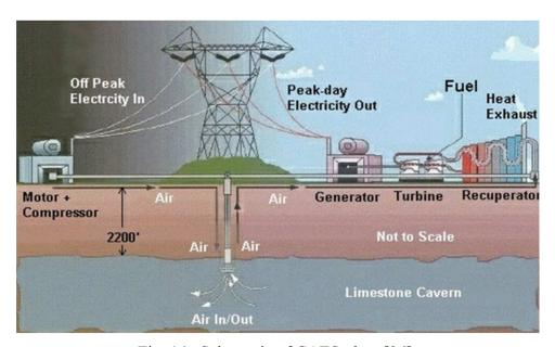
Fig. 14. Schematic of CAES plant [36].
