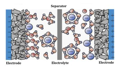
Fig. 12. Individual supercapacitor cell [19].
