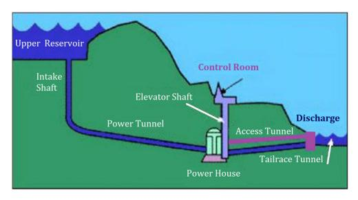
Fig. 13. Schematic of Pumped Hydro Storage plant [34].
