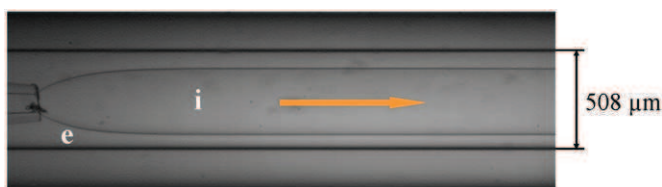
Fig. 3. Picture of the annular flow in a PFA tube where (i) is the internal fluid (sunflower oil) and (e) the external fluid (EtONa/EtOH solution).
