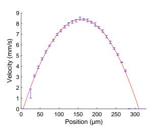
Fig. 5 A comparison between theoretical profile (solid red curve) and 8 consecutive measured profiles (blue errorbars) along the centre-line of the flow channel with a flow speed of 20  $\mu$ L/min<sup>-1</sup>. The liquid is milk (2 %) diluted in water
