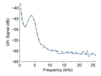
**Fig. 3** OFI signal in frequency domain measured at the middle of the channel and the corresponding fitting curve (Eq. (6)). The mean frequency in the sensing volume is calculated by extracting the Doppler frequency of the signal
