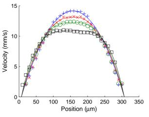
Fig. 8 Measured (markers) and theoretical (solid line) velocity profile in a 320  $\mu$ m channel for various solutions of xanthan gum (0 (plus), 0.25 (cross), 1 (circle), and 3 g/L (square))
