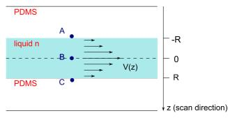
Fig. 2 Diagram showing the scan configuration with respect to the zaxis of the flow channel. The angle calibration is calculated at position B, and the velocity profile is measured from A to C. The flow channel has a 160 µm internal radius R
