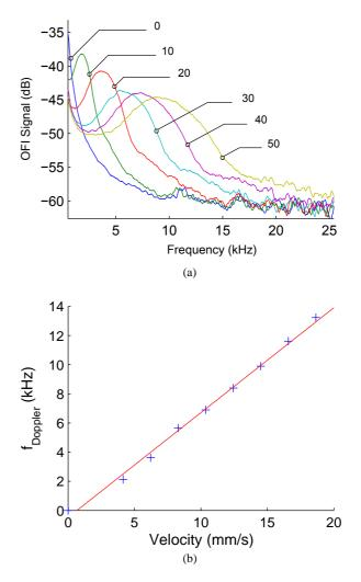
**Fig. 4** (a) OFI signal in the frequency domain for several flow rates (0, 10, 20, 30, 40 and 50  $\mu$ L.min<sup>-1</sup>) (b) Plot of the Doppler frequency as a function of the flow rate. The peak frequency shows a linear relationship with velocity. The angle between the flow direction and the optical beam can be estimated from the slope of this relationship, and has been calculated to be 80.25 °
