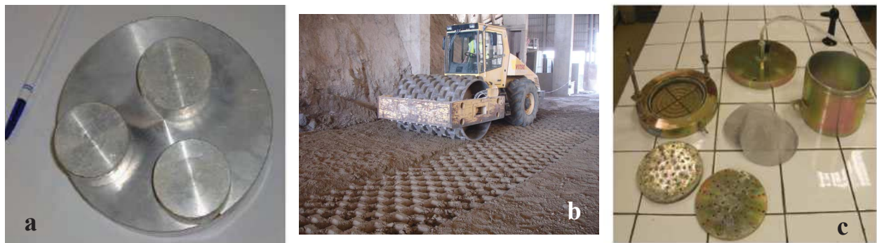
Figure 1: Kneading compaction tool for laboratory tests (a) simulating the sheepfoot roller compaction (b), and permeameter (c).
