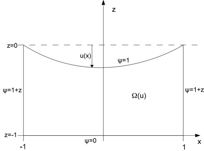
FIGURE 1. Idealized electrostatic MEMS device.
