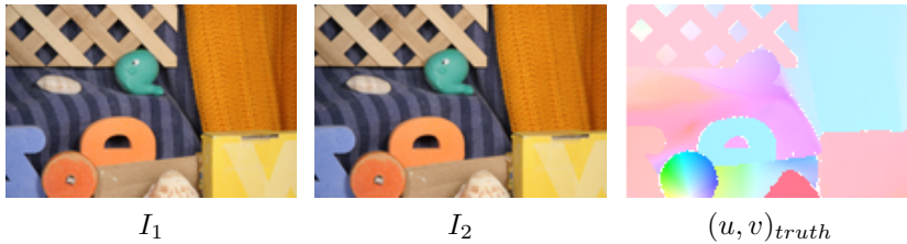
FIG. 6.4. Images I_1 and I_2 of the RubberWhale sequence. The optical flow ground truth is presented, the color representing the direction of the flow, while the intensity is related to the norm of the vector.
