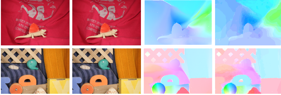
FIG. 6.7. Results obtained with the non convex approach on the Middlebury data Dimetrodon and Rubberwhale. The original images are shown in the first and second columns. The true optical flow in the third column is then compared to the estimated one in the fourth.
