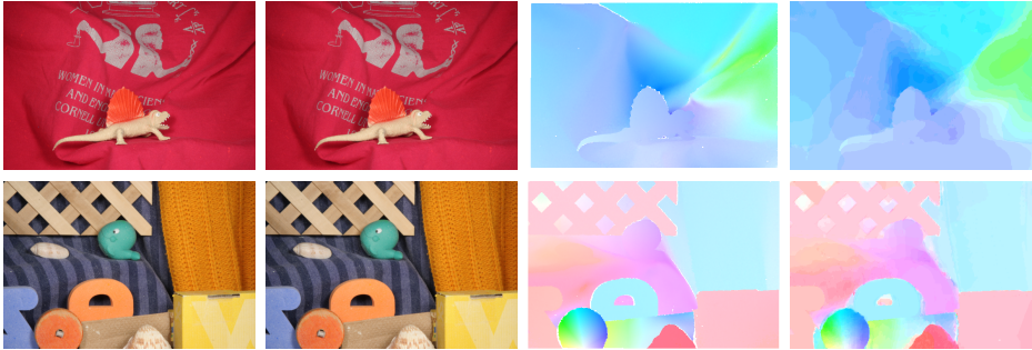
FIG. 6.7. Results obtained with the non convex approach on the Middlebury data Dimetrodon and Rubberwhale. The original images are shown in the first and second columns. The true optical flow in the third column is then compared to the estimated one in the forth.
