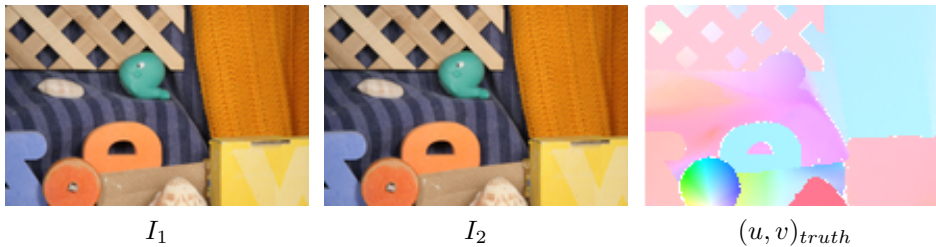
FIG. 6.4. Images I_1 and I_2 of the RubberWhale sequence. The optical flow ground truth is presented, the color representing the direction of the flow, while the intensity is related to the norm of the vector.
