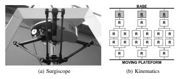
Figure 2. Surgiscope kinematics.
