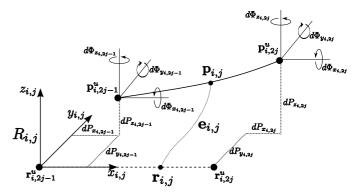
Figure 1. Notation associated with each beam  $B_{i,j}$ .
