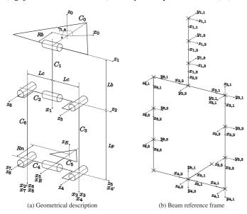
Figure 3. Kinematic chain description.
