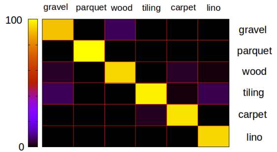
Fig. 6. Confusion matrix obtained for ground classification with 6 ground types. The error rates obtained for the ground types of gravel, parquet, wood, tiling, carpet and lino are, respectively, 9%,6%,2%,4% and 6%.
