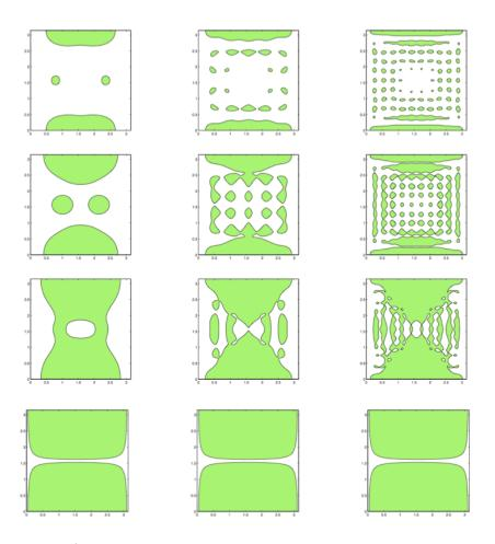
Figure 7:  $\Omega = (0, \pi)^2$ , with Dirichlet boundary conditions on  $\partial\Omega \cap (\{x_2 = 0\} \cup \{x_2 = \pi\})$  and Neumann boundary conditions on the rest of the boundary. Row 1: L = 0.2; row 2: L = 0.4; row 3: L = 0.6; row 4: L = 0.9. From left to right: N = 2 (4 eigenmodes), N = 5 (25 eigenmodes), N = 10 (100 eigenmodes).
