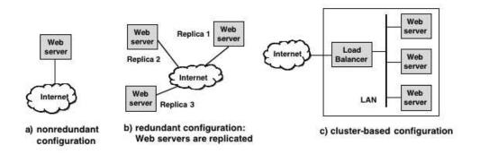
Fig. 6. Example of configurations for a Web server
