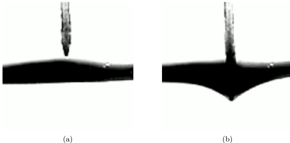
Fig. 2: The left image shows the situation before the needle moved into the colored gelatine layer visible as a black horizontal bar (a). The right image illustrates the maximum deformation of the layer, this defines the endpoint for the measurements (b). The distance between the lower boundary of the layer in (a) and the needle tip in (b) is measured as an estimate for the deformation, it is approximately 3.28 mm.
