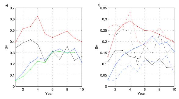
**Figure 15.** Mean annual volume transport anomaly (Sv) through (a) the CAA and (b) Lancaster Sound (dashed line) and Smith Sound (solid line with dots) in experiments WIND (black), FLUX (blue), NAO (red), and, in Figure 15a, FLUX ATL (green).
