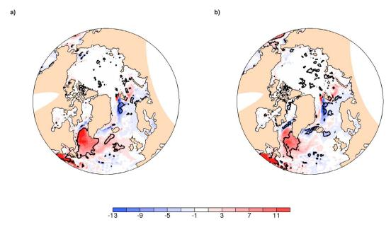
**Figure 12.** The (a) 1 year lagged (heat flux leads) and (b) simultaneous regressions of the mean annual surface heat flux (W m<sup>-2</sup>) on the annual SSH in Smith Sound. The bold black contour indicates the 95% level of significance.
