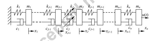
Figure 1 The MDOF structural system considered in the present study
