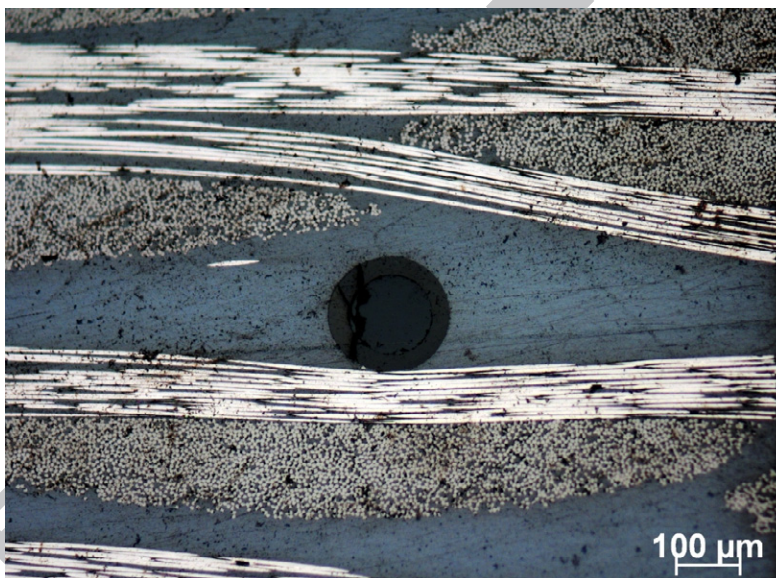
Figure 5. a, b) Cross-sectional view of composite along the length of the optical fibre.
