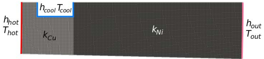
Figure 7: Schematic of a regeneratively cooled rocket engine combustion chamber. The drawings are not to scale.
