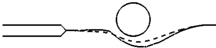
Figure 9: Comparison of crack paths obtained via adaptive cohesive model (plain line) and linear elastic fracture mechanics (dashed).
