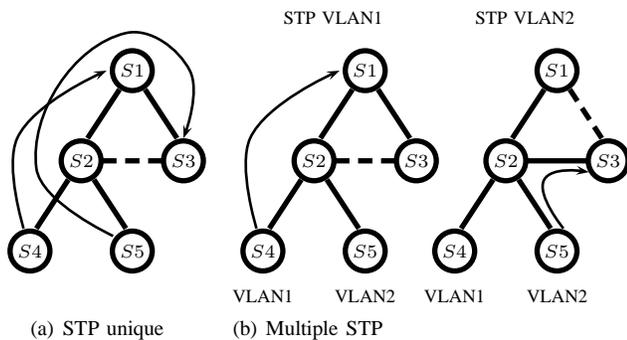
FIGURE 8. Configuration STP unique vs Multiple STP
