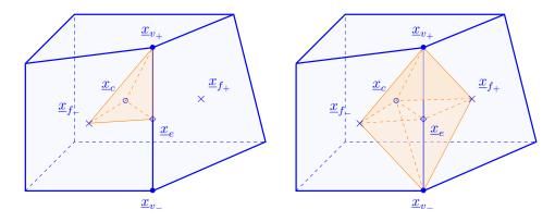
Figure 4: Left: barycentric subdivision of a primal cell with an elementary subsimplex highlighted ( $\underline{x}_c$  is not necessarily the barycenter of c); Right: elementary subvolume considered for the gradient reconstruction in the Discrete Geometric Approach.
