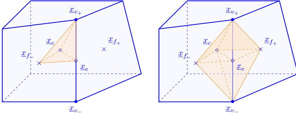
Figure 4: Left: barycentric subdivision of a primal cell with an elementary subsimplex highlighted ( $\underline{x}_c$  is not necessarily the barycenter of  $c$ ); Right: elementary subvolume considered for the gradient reconstruction in the Discrete Geometric Approach.
