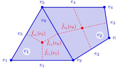
Figure 3: Geometric entities for local discrete Hodge operator.
