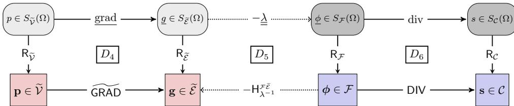
Figure 5: Tonti diagrams for the exact problem and the cell-based scheme (15).
