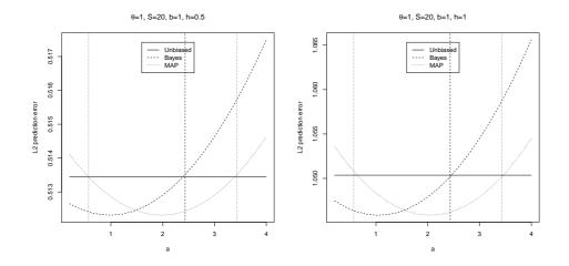
FIGURE 1.  $L^2$  prediction error for  $\theta = 1$  in terms of a with  $\Gamma(a, 1)$  prior: UP (plain horizontal), BP (dashes), MAP (dots) for S = 20. Vertical lines corresponds to  $a = 1 + \sqrt{S^{-1} + 2}$  (dashes) and  $a = 2 \pm \sqrt{S^{-1} + 2}$ (dots). On the left : h = 0.5, on the right : h = 1.
