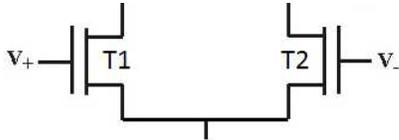
Fig. 13. Differential Pair Schematic View.
