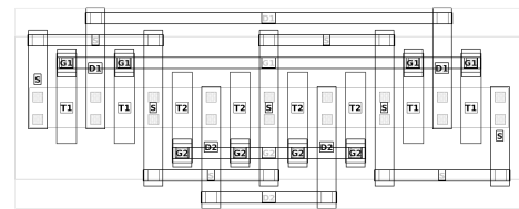
Fig. 13. Differential Pair (mirror layout style) 65nm
