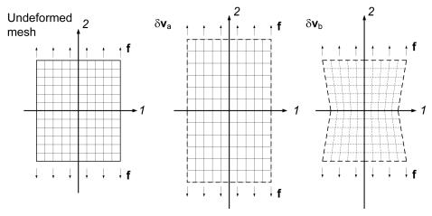
Fig. 12 Schematic view of the adopted virtual fields  $\delta \mathbf{v}_a$  and  $\delta \mathbf{v}_b$  illustrated as deformation of a regular mesh.
