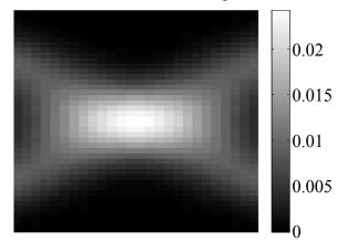
Fig. 16 Contour plot of the strain increment component  $\Delta E_{22}$  at the test time t=0.70 obtained using the convolutions method. In the left plot 5 time steps have been used to compute the strain increment, in the right plot 15 time steps.
