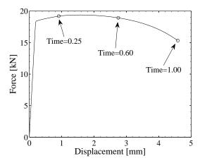
Fig. 4 Force vs displacement curve obtained from the simulated tests. The maximum imposed displacement is  $4.6~\mathrm{mm}$  which correspond to the reference time  $t{=}1.00$ .
