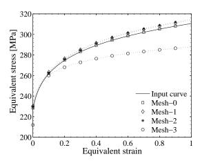
Fig. 14 Comparison of the stress-strain curves obtained with the parameter identified using different measurement meshes.
