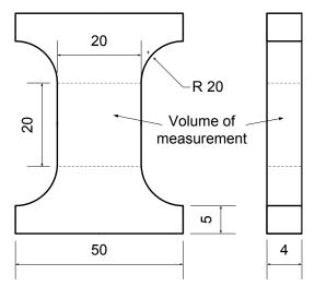
Fig. 1 Geometry of the specimen used in the simulated test (dimensions in mm). The three dimensional displacement field used in the identification procedure is the one inside the volume of measurement.
