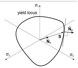
Fig. 9 Representation of a general yield locus in the Haigh-Westergaard plane. The normalised tensors  $\hat{\mathbf{N}}_S$  and  $\hat{\mathbf{N}}_p$  represent the direction of the deviatoric stress and the direction of the plastic flow respectively.
