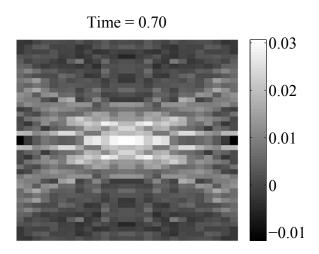
**Fig. 15** Contour plot of the strain increment component  $\Delta E_{22}$  at the test time t=0.70 in the central section of the volume of measurement. The effect of the introduced noise is clearly visible.
