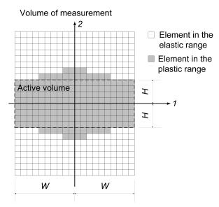
Fig. 10 Definition of the active volume. The computation of the cost function is restricted to the zone of the volume of measurement, called the *active volume*, in which all the elements are subjected to plastic deformation.
