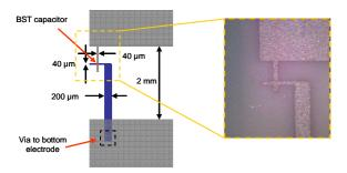
Figure 9. Detail of the ferroelectric capacitor.
