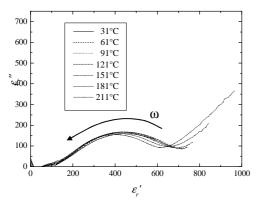
Figure 2. Argand diagramm representation ( $\varepsilon_r$ " vs  $\varepsilon_r$ ) of Ba<sub>0.90</sub>Sr<sub>0.10</sub>TiO<sub>3</sub> thin films dopes with 1% manganese for different temperatures.
