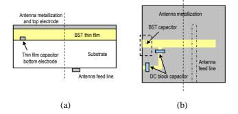
Figure 7. Schematic cross section view (a) and top view (b) of the BST thin film notch antenna.
