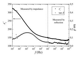
Figure 5. Dielectric permittivity  $\varepsilon_i$  and losses tan  $\delta$  as a function of frequency of a PbZr<sub>0.57</sub>Ti<sub>0.43</sub>O<sub>3</sub> thin film.
