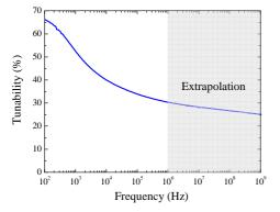
Figure 6. Etrapolation to the UHF frequency region of the tunability of  $$Ba_{0.80}Sr_{0.20}TiO_3$ thin films.}$
