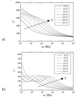
Figure 1. Real part  $\varepsilon_r^{,*}$  (a) and imaginary part  $\varepsilon_r^{,*}$  (b) of the complex dielectric permittivity of Ba<sub>0.90</sub>Sr<sub>0.10</sub>TiO<sub>3</sub> thin films dopes with 1% manganese as a function of frequency and at different temperatures.
