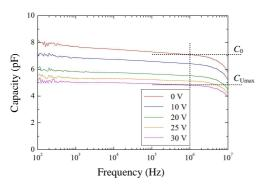
Figure 10. Capacity – frequency dependency of the integrated BST varactor for different DC bias voltage.
