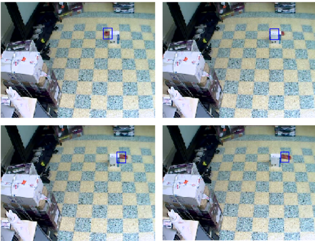
Fig. 8: Kalman Filter with mean-shift algorithm to overcome the total occlusion problem.
