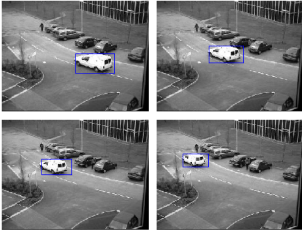
Fig. 3: Tracking using an adaptive scale for the ROI
