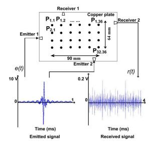
FIG. 1. (Color online) Training step of the disturbed acoustic diffraction tactile process on a copper plate. 32 × 36 predefined positions are sequentially touched by an index; received reference signals from two PZT transducers are stored according to the contact positions.
