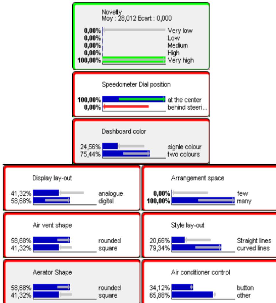
Figure 12 The optimal technical choices designer should carry out in order to improve the novelty perception of a dashboard. Compared to Figure 11, this model allows identifying all technical choices and not only the most relevant. Hence, it provides designer with more flexibility and choice possibilities.
