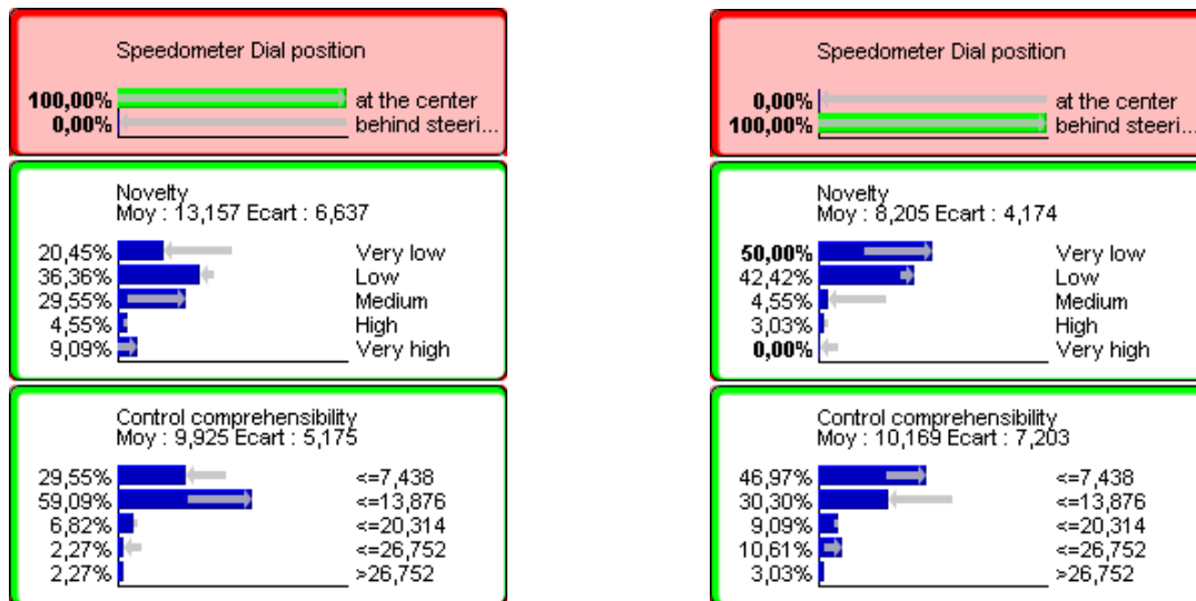
Fig. 5. The influence of the speedometer dial position on the dashboard novelty lay out as well as on the control comprehensibility: a dashboard whose speedometer dial is located at the center is perceived by customers as more novel than a dashboard whose speedometer dial is located behind the steering wheel. However, that choice may deteriorate the control comprehensibility.
