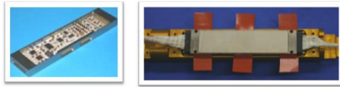
Figure 17: The PEC "HPHT" Concept. Left side: Open casing with the substrate and electronic components inside. Right side: The integrated box (I) technical solution for the chassis.
