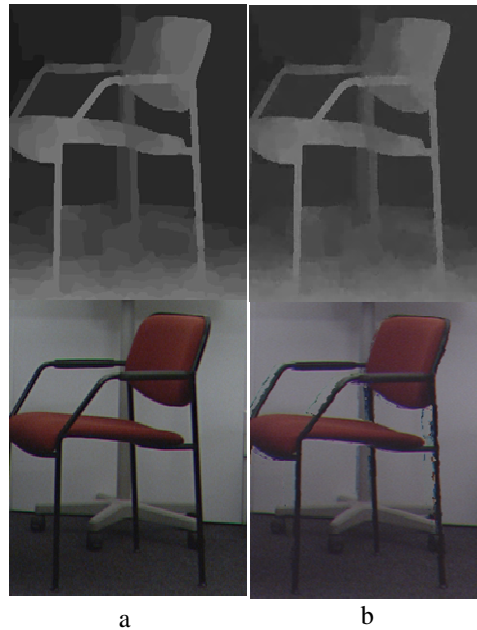
Figure 4: Ringing artifacts in depth data lead to distortions in the synthesized views. a: Original depth frame (up) and original color frame (bottom). b: Distorted depth frame (up) and synthesized frame (bottom).
