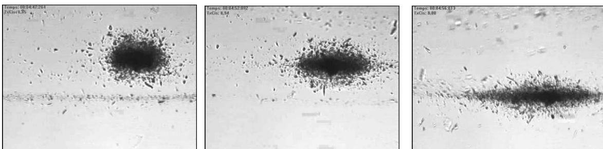
Figure 7: Shearing of an individual agglomerate at 9 \text{ s}^{-1} and times 0 s, 4.8 s, 8.72 s (Image width is 500 \mu\text{m} ).
