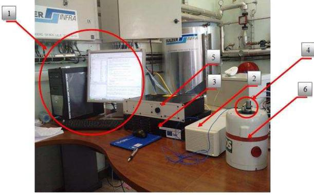
Fig. 2. Picture of the shaker and of the recording system. 1: Computer, 2: dSPACE, 3: conditioner, 4: accelerometer, 5: preamplifier, 6: shaker.
