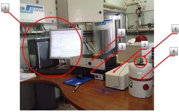
Fig. 2. Picture of the shaker and of the recording system. 1: Computer, 2: dSPACE, 3: conditioner, 4: accelerometer, 5: preamplifier, 6: shaker.
