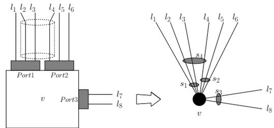
**Figure 1: An example of localized risks. Link  $l_4$ , for instance, shares risk  $s_2$ , corresponding to Port 2 failure, with  $l_5$  and  $l_6$  and shares risk  $s_4$ , corresponding to the conduit cut, with links  $l_2$  and  $l_3$ .**
