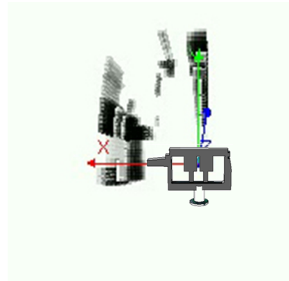
(b) BVM results for binaural processing only. Interpretation, from left to right: 1) sound coming from speaker triggers an estimate for occupancy from the binaural sensor model, and a consecutive exploratory gaze shift at approximately 1.6 seconds; 2) At approximately 10 seconds, noise coming from the background introduce a false positive, that is never again removed from the map (i.e. no sound does not mean no object, only no audible sound-source).
