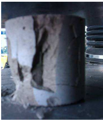
Figure 1: Pattern failure of samples under uniaxial compression and three points bending tests device
