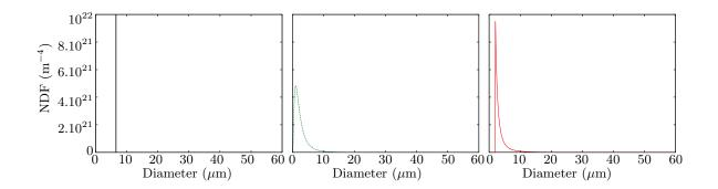
Fig. 2 Different number density functions (NDF) with the same total bulk density and average diameter  $d_{31}$  – Left: Dirac size distribution (monodisperse); Middle: lognormal size distribution; Right: window size distribution.
