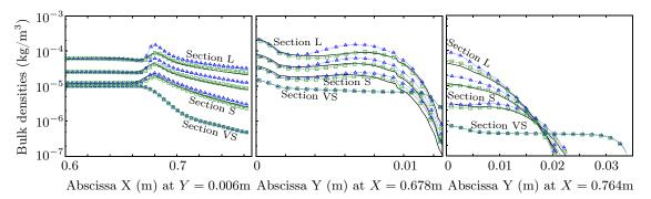
Fig. 20 Droplet mass concentrations along cuts (left: cut A-A, middle: cut B-B, right: cut C-C) – Solid: MF-PEG reference (BWC, 1 curve for each of the 3 sections);  $\Delta$ : MF BWC;  $\Box$ : MF ACS. Compared to MF-PEG, the MF solutions have 1 more curve for the section of VS droplets.
