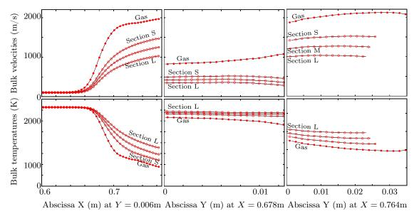
Fig. 19 Velocities and temperatures along cuts (left: cut A-A, middle: cut B-B, right: cut C-C) – Solid: MF-PEG BWC (reference); •: MF-PEG ACS – Empty symbols: disperse phase (per section); Filled symbols: gas.
