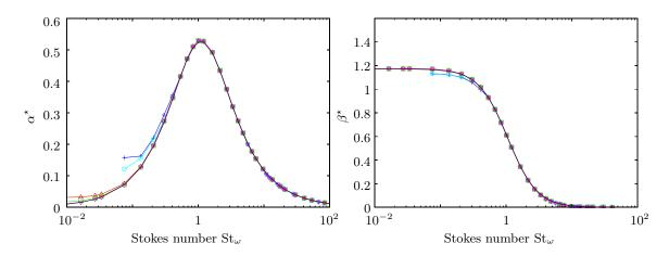
Fig. 10 Attenuation and dispersion of a monochromatic wave in a monodisperse spray with C = 0.106 for different coupling time steps (SAP1 code,  $K_p = 0.25$ ) – Line: analytic; +:  $K_g = 2$ ;  $\circ: K_g = 1$ ;  $\Delta: K_g = 0.9$ ;  $\Box: K_g = 0.5$ ;  $\nabla: K_g = 0.2$ .
