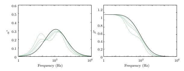
Fig. 27 Attenuation  $\alpha^*$  and dispersion  $\beta^*$  of a monochromatic acoustic wave in a polydisperse lognormal spray – Dotted: MF with 2, 3, 4, and 10 sections with Fixed mass  $\Delta r$  discretization method; Solid: reference.
