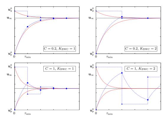
Fig. 7 BWC computation of a 0D gas-droplet relaxation case for different mass loadings and different  $K_{BWC} - A$ : gas; •: droplets; Line: exact solution for each phase.
