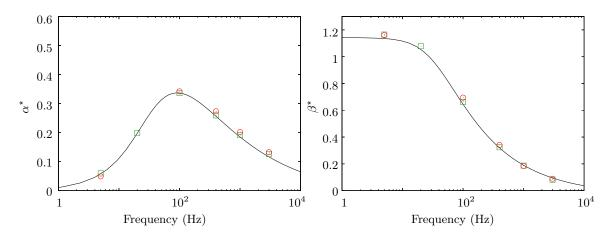
Fig. 15 Attenuation and dispersion of a monochromatic acoustic wave in a polydisperse spray – Line: analytic;  $\Box$ : SAP1 (ACS splitting, 10 sections);  $\circ$ : CEDRE (ACS splitting, 10 sections).
