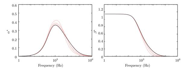
Fig. 5 Attenuation  $\alpha^*$  and dispersion  $\beta^*$  of a monochromatic acoustic wave in a polydisperse window spray – Dotted: MF with 2, 3, 4, and 10 sections with constant  $\Delta r$ ; Solid: reference.
