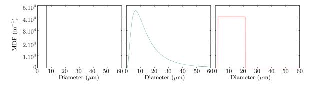
Fig. 3 Different mass density functions (MDF =  $4/3\pi r^3$ NDF) with the same total bulk density and average diameter  $d_{31}$  – Left: Dirac size distribution (monodisperse); Middle: lognormal size distribution; Right: window size distribution.
