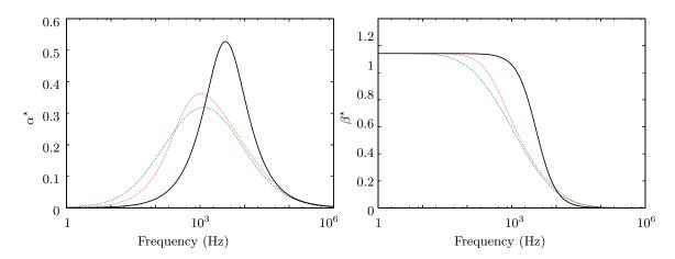
Fig. 4 Attenuation  $\alpha^*$  and dispersion  $\beta^*$  of a monochromatic acoustic wave in a polydisperse spray – Solid: Dirac size distribution (monodisperse); Dotted: window size distribution; Dashed: lognormal size distribution.
