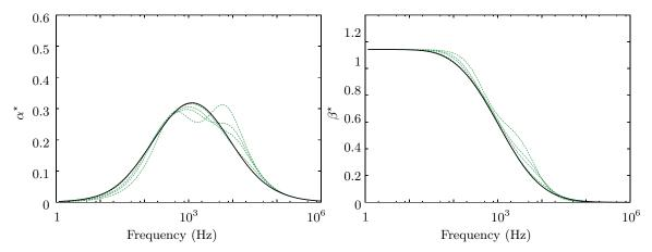
Fig. 6 Attenuation  $\alpha^*$  and dispersion  $\beta^*$  of a monochromatic acoustic wave in a polydisperse lognormal spray – Dotted: MF with 2, 3, 4, and 10 sections with Fixed mass  $\Delta r$  discretization method and exact  $r_{31}$ ; Solid: reference.
