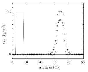
Fig. 11 Convection of a droplet structure with a time step driven by acoustics (window packet convected at 30m/s, second order Bouchut scheme, SAP1 code) – + droplet phase transport at  $CFL_k = 0.081$ ; × droplet phase transport at  $CFL_k = 0.94$ ; —: initial state.
