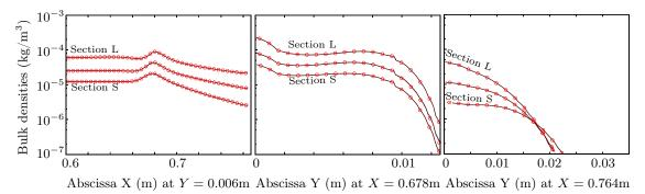
Fig. 18 Droplet mass concentrations along cuts (left: cut A-A, middle: cut B-B, right: cut C-C) – Solid: MF-PEG BWC (reference); o: MF-PEG ACS.
