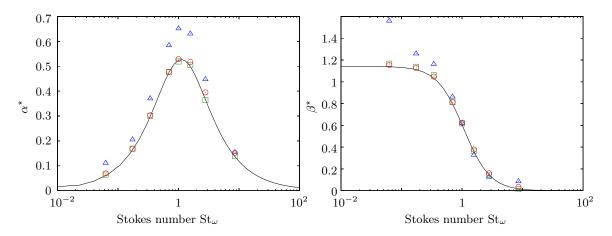
Fig. 14 Attenuation and dispersion of a monochromatic acoustic wave in a monodisperse spray with C = 0.106 – Line: analytic;  $\Delta$ : CEDRE (BWC technique);  $\Box$ : SAP1 (ACS splitting);  $\circ$ : CEDRE (ACS splitting).
