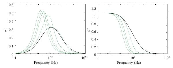
Fig. 24 Attenuation  $\alpha^*$  and dispersion  $\beta^*$  of a monochromatic acoustic wave in a polydisperse lognormal spray – Dashed: MF with 2, 3, 4, 10, and 100 sections with constant  $\Delta S$ ; Solid: reference.
