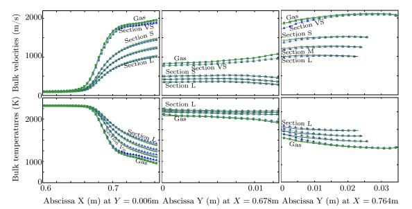
Fig. 21 Velocities and temperatures along cuts (left: cut A-A, middle: cut B-B, right: cut C-C) – Solid: MF-PEG reference (BWC);  $\Delta$ : MF BWC;  $\Box$ : MF ACS – Empty symbols: disperse phase; Filled symbols: gas. Compared to MF-PEG, the MF solutions have 1 more curve for the section of VS droplets, which is almost superimposed to that of the gas, given the fast time scales of VS droplets.
