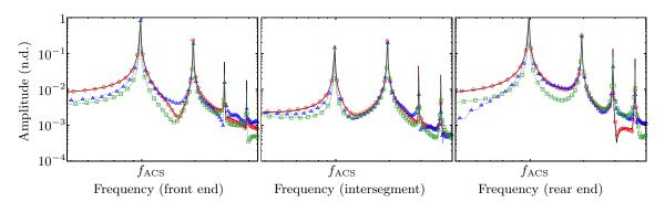
Fig. 22 Spectra of pressure signal non dimensioned by the ACS highest peak – Left: front-end sensor (1); Middle: middle sensor (2); Right: rear-end sensor (3) – Solid: MF-PEG BWC (reference);  $\circ$ : MF-PEG ACS;  $\Delta$ : MF BWC;  $\Box$ : MF ACS.
