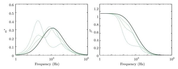
Fig. 26 Attenuation  $\alpha^*$  and dispersion  $\beta^*$  of a monochromatic acoustic wave in a polydisperse lognormal spray – Dotted: MF with 2, 3, 4, and 10 sections with Geometric discretization method; Solid: reference.
