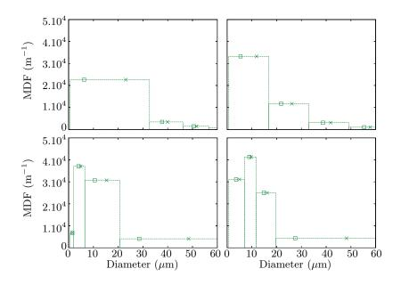
Fig. 23 Four methods of discretization/reconstruction for the lognormal distribution using 4 sections; - - - section bounds with area proportional to mass;  $\times$ :  $d_{31}$  computed with  $\kappa(r) = cst$ ;  $\Box$ : exact  $d_{31}$  – Top Left: Constant  $\Delta S$  discretization method; Top Right: Constant  $\Delta r$  discretization method; Bottom Left: Geometric discretization method; Bottom Right: Fixed mass  $\Delta r$  discretization method.
