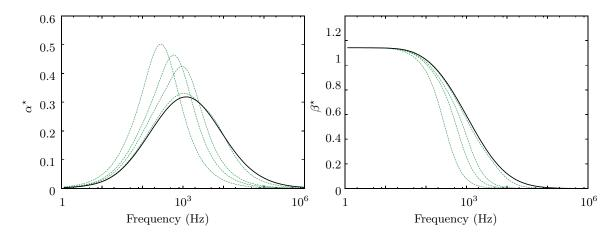
Fig. 25 Attenuation  $\alpha^*$  and dispersion  $\beta^*$  of a monochromatic acoustic wave in a polydisperse lognormal spray – Dotted: MF with 2, 3, 4, and 10 sections with constant  $\Delta r$ ; Solid: reference.
