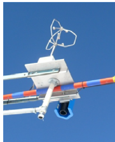
Figure 2: Ultrasonic anemometer and snow depth sensor (Jenoptik)
