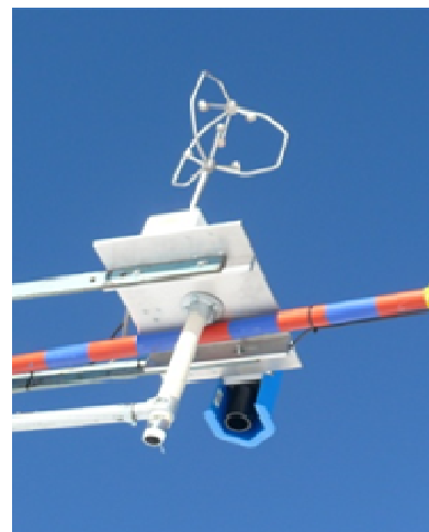
Figure 2: Ultrasonic anemometer and snow depth sensor (Jenoptik)
