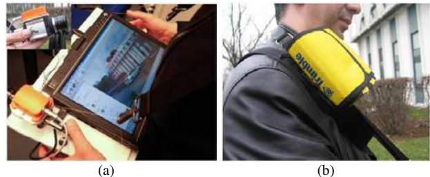
Fig. 1. Hardware platform of Raxenv Project. (a) Tablet PC, camera and inertial sensor (b) GPS receiver.
