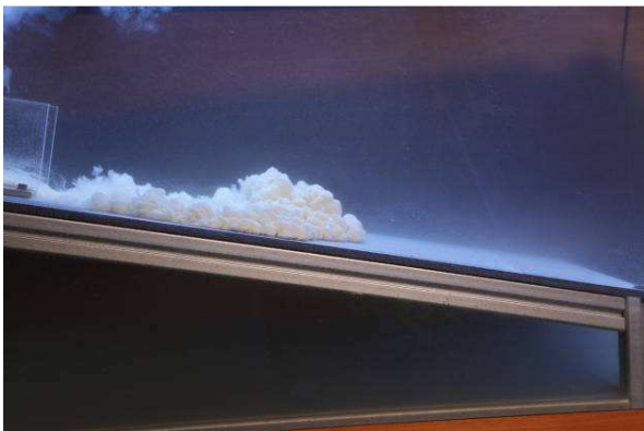
Photos 21, 22: "Very" small-scale modeling of powder avalanche (by courtesy of Isabelle Ousset)
